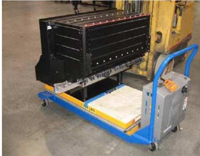
Figure 2.1: Tesla Roadster battery pack, from [7].
