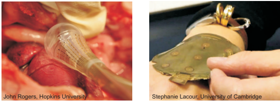
Figure 1: Stretchable electronics examples. Left: heart ablation catheter. Right: Electronic skin for wearable mobile phone.
