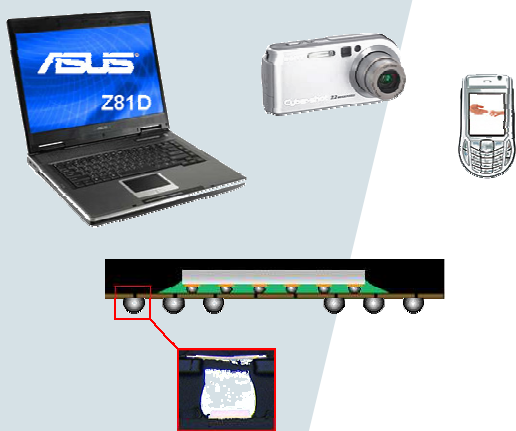
Figure 1 Commercial electronic products, BGA cross section and a failed solder bump.
