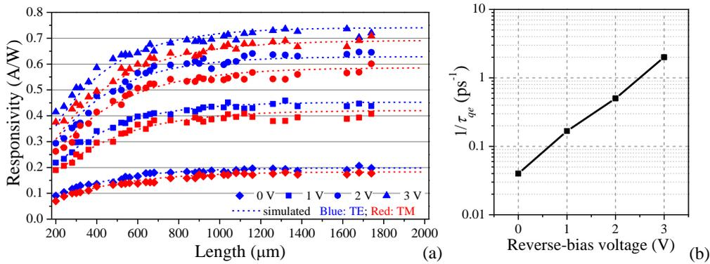
Fig. 2 (a) The measured and simulated responsivities of devices with the lengths ranging from 200  $\mu\text{m}$  to 2000  $\mu\text{m}$  at a wavelength of 1640 nm. The measurements and simulations are done under four different reverse-bias voltages and for both polarizations. (b) The  $\tau_{qe}$  at different reverse-bias voltages.
