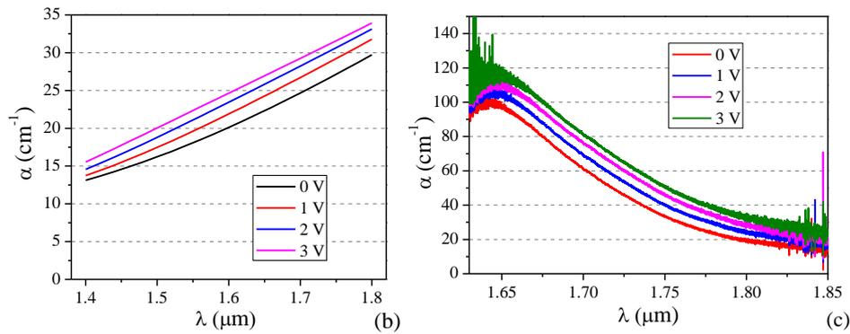
Fig. 3 (a) The spectral simulations of a 960  $\mu\text{m}$ -long device for TE polarization. The measured spectra are also shown for comparison. (b) The total photon absorption of the QDs calculated by the rate equation model (for TE polarization). (c) The measured absorption spectra for different reverse-bias voltages (for TE polarization, including pure propagation loss of the optical mode).
