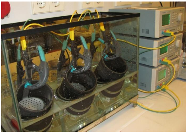
Fig. 1: RCM test set – up
