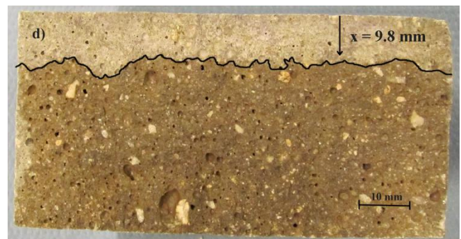
Fig. 2: Examples of chloride penetration depths revealed by \text{AgNO}_3 solution applied onto freshly split mortars after RCM test – a) OPC-mortar, b) GGBS-mortar, c) FA-mortar, d) SF-mortar
