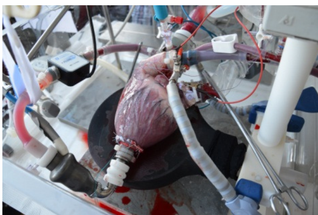
Figure 1 Experimental set-up of the ex vivo porcine heart model supported with a Heartmate II VAD. A similar set-up was used for the measurements on the hearts supported with a Micromed DeBakey VAD.
