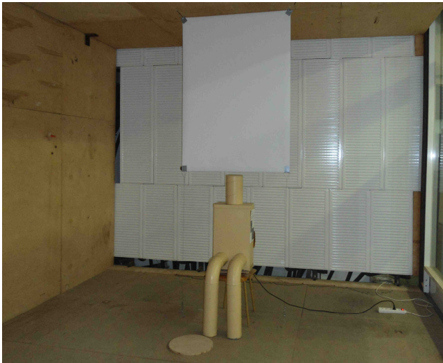
Fig. 2 Experimental chamber with thermal manikin
