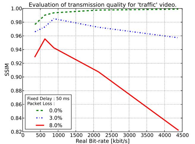
Fig. 6. The effect of a gradually increased bit-rate on the streaming of "traffic" video. Snapshots on three values of packet loss.
