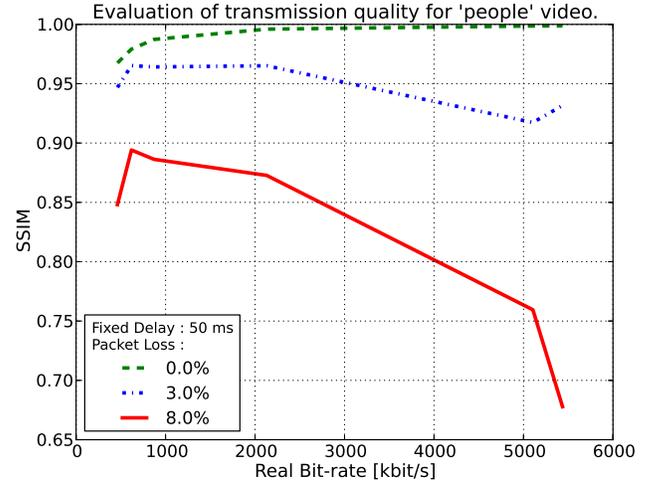
Fig. 5. The effect of a gradually increased bit-rate on the streaming of "people" video. Snapshots on three values of packet loss.
