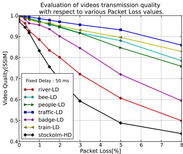
Fig. 4. The effect of packet loss on seven streamed videos, 6 in low definition format (LD) and 1 in high definition format (HD).
