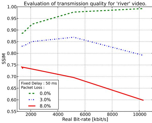
Fig. 7. The effect of a gradually increased bit-rate on the streaming of "river" video. Snapshots on three values of packet loss.
