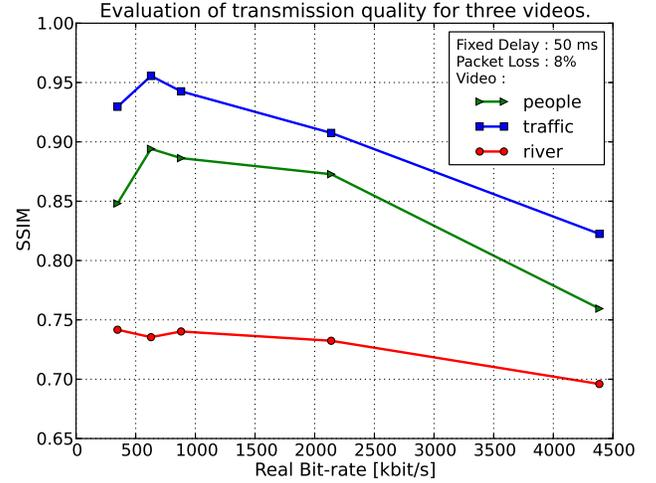
Fig. 8. Comparison of the effects yield by a gradually increased bit-rate on the streaming of three videos with fixed packet loss of 8%.
