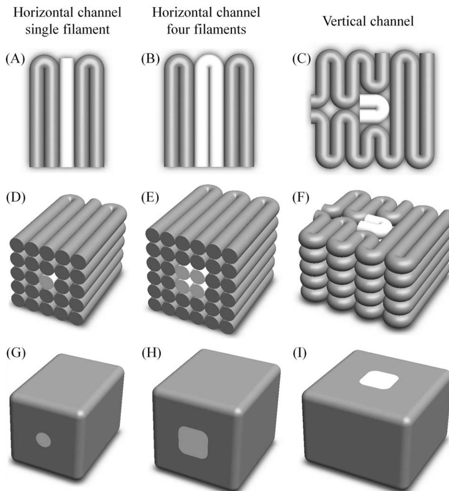
**FIGURE 1.** Schematic representation of the three different channels in bulk material: (A,D,G): horizontal channel consisting of a single filament; (B,E,H): horizontal channel consisting of four filaments and (C,F,I): vertical channel. (A–C) show the third layer of the printed construct indicating the printing path of both phases; (D–F) show the 3D objects indicating the printing path and amount printing layers per object and (G–I) show the 3D object with the channel as second phase.
