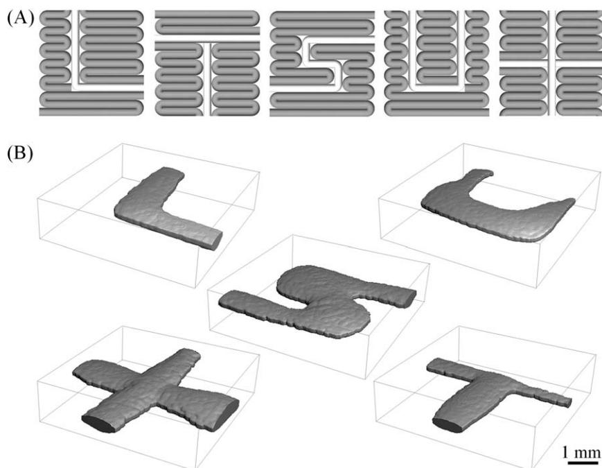
**FIGURE 6.** (A) schematics of different channel geometries embedded in the bulk material. (B) negative  $\mu$ CT images of the 3D printed hydrogel constructs. The outer dimensions of the investigated volume of interest are indicated with the box.
