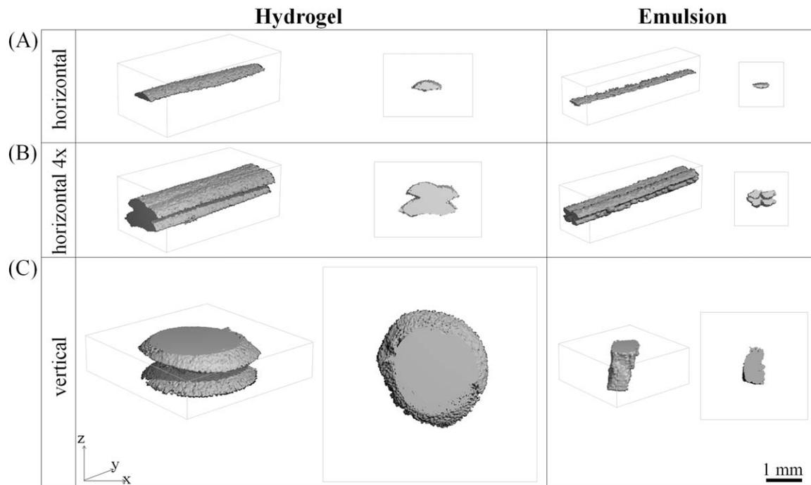
**FIGURE 3.** Negative images of printed channels in bulk material. The left column shows representative samples printed with hydrogel and the right column shows representative samples printed with emulsion. Row (A) shows the horizontal channels consisting of a single filament in bulk material, row (B) the horizontal channels consisting of four filaments in bulk material and row (C) the vertical channels in bulk material.
