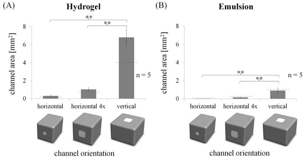
**FIGURE 4.** Theoretical ( $A_t$ ) and printed ( $A_p$ ) channel cross-sectional area of (A) the hydrogel and (B) the emulsion.  $A_t$  is illustrated with a dashed line;  $A_p$  is illustrated as column and indicated as means  $\pm$  standard deviation with  $n = 5$ .  $*p < 0.05$ ,  $**p < 0.01$ . The values correspond to  $A_t$  and  $A_p$  from Table I.
