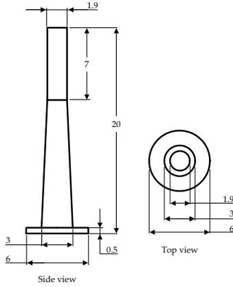
Figure 1. Dimensions of the dielectric rod. All the dimensions are in millimeter.
