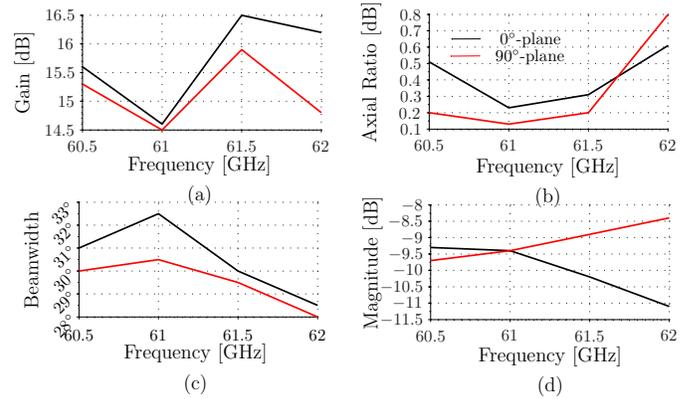
Figure 10. Measured antenna performance over the frequency band of interest (i.e. (-20dB) isolation bandwidth from 60.45 - 61.55 GHz). (a) Co-polarization gain, (b) Axial ratio, (c) 3dB beamwidth, and (d) SLL.
