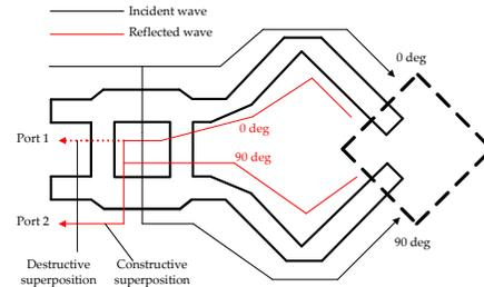
Figure 4. Illustration of the essential paths with their relative phases that cause the interchanged scattering parameters (with the assumption that the system is more antenna-limited than coupler-limited).
