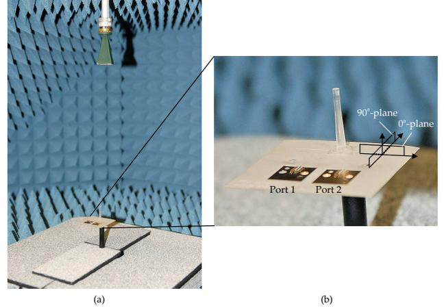
Figure 6. (a) The 60-GHz anechoic chamber and (b) the dielectric rod antenna.
