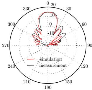
Figure 8. RHCP radiation patterns in the  $90^\circ$ -plane at 61 GHz.
