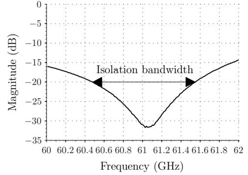
Figure 9. Definition of (-20dB) isolation bandwidth from  $S_{21}$  measurement. Note that -20dB isolation means -20dB coupled to port 2.
