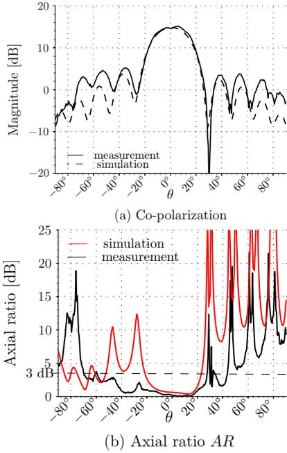
Figure 7. Radiation patterns in the  $0^\circ$ -plane at 61 GHz for (a) Co-polarization pattern (with achieved 14.6dBi gain) and (b) axial ratios in the  $0^\circ$ -plane
