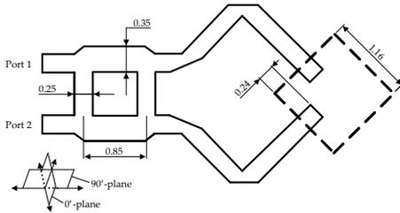
Figure 2. Dimensions of the quadrature hybrid coupler and patch antenna. All the dimensions are in millimeter.
