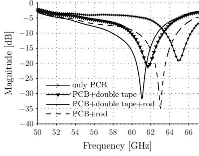
Figure 5. Measured  $S_{21}$  for step-wise integration of the patch antenna and dielectric rod.
