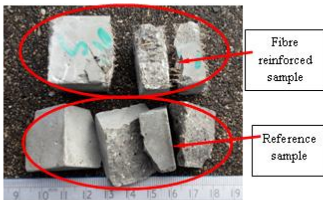
Fig. 5 Fractions of the samples (fibre reinforced and plain samples) after Charpy impact test
