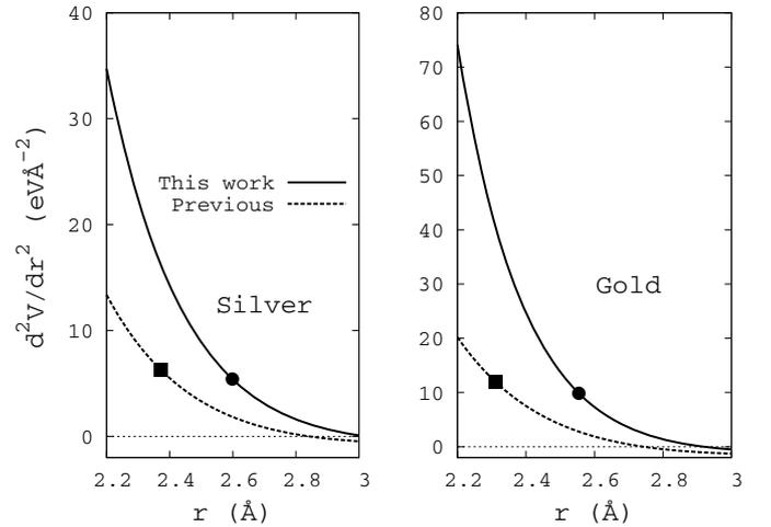
**Fig. 5.** The second derivative of the Ag<sub>2</sub> and Au<sub>2</sub> dimer potentials. Our results are shown as full lines while previous parameterizations [41–43] are shown as dashed lines. The points locate the curvature at the corresponding equilibrium distances.
