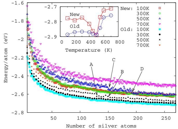
**Fig. 8.** The evolution of the energy per atom vs. Ag cluster size at different deposition temperatures. Open symbols: new parameters, closed symbols: old [43]. The arrows indicate points of energy drops. Inset: temperature dependence of  $e_{\infty}$  (see Eq. (9)).
