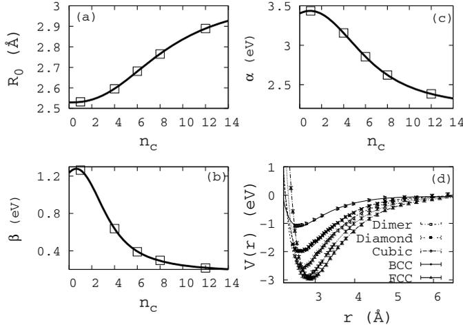
**Fig. 3.** DFT parameters of the Gupta potential for the four phases of Ag: FCC, BCC, simple cubic, diamond-like phase and dimer. The fitted potentials are shown in panel (d) and the points are the corresponding DFT binding energies.
