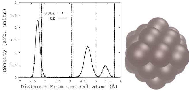
**Fig. 7.** Left: density distribution as a function of distance from the central atom of a  $\text{Ag}_{55}$  cluster for the unrelaxed (thin-dotted line) and the MD-relaxed structure at 300 K (full line). The feature at 4.09 Å in the unrelaxed cluster shifts upwards and merges with the feature at 5.0 Å which shifts downwards. Right: snapshot of MD-relaxed cluster at the end of the 2 ns simulation.
