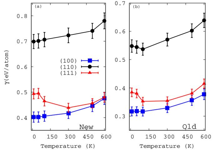
**Fig. 6.** The surface energy per atom for current and previous parameters for (100)-(rectangle), (110)-(circle) and (111)-(triangle) oriented silver surfaces at low temperature. The results of the current work are on the left panel (a) and those of previous [43] are in panel (b).
