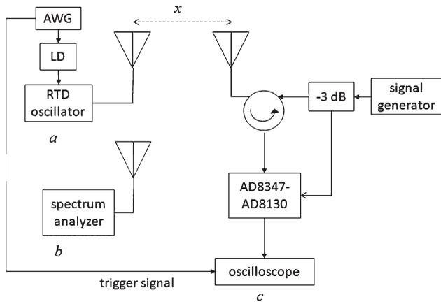
**Figure 2** Diagram of wireless interrogation system elements ( $x \sim 30$  cm). (a) Optically modulated RTD-based oscillator attached to antenna. (b) Auxiliary antenna used for wireless monitoring of signal locking. (c) Locking signal transmitter and wireless received signal demodulator
