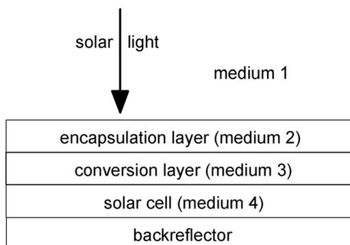
FIG. 1. Schematic overview of the solar cell (medium 4) with a conversion layer (medium 3), encapsulation layer (medium 2) and a back-reflector, surrounded by air (medium 1).
