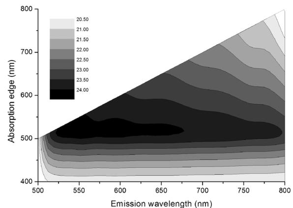
FIG. 6. Calculated efficiencies of a CdTe solar with a spectral shifting layer as a function of the absorption edge  $\lambda_a$  and the emission wavelength  $\lambda_{\text{em}}$ .
