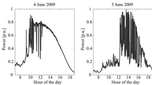
**Fig. 1** Solar power measured on 4th June and 5th June from TU Delft 12.6 kW photovoltaic array
