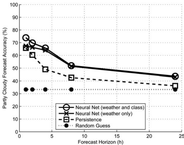
**Fig. 7** Forecast accuracy for partly cloudy conditions against horizon for three forecasting methods
