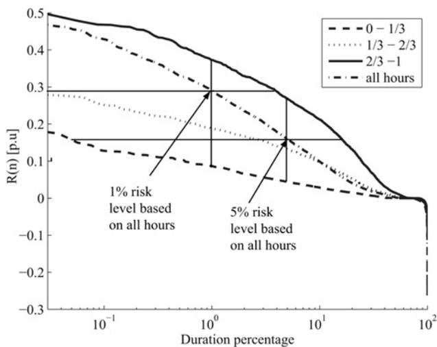
**Fig. 4** Sorted curve of upward reserves  $R(n)$  based on aggregated fluctuations of eight sites in the Netherlands, for all hours (dash-dot) and for periods having increasing fractions of partly cloudy sites (dotted, dashed, solid). Cross hairs indicate variable risk of fixed reserve (horizontal hair) and variable reserve necessary for fixed risk (vertical hair).
