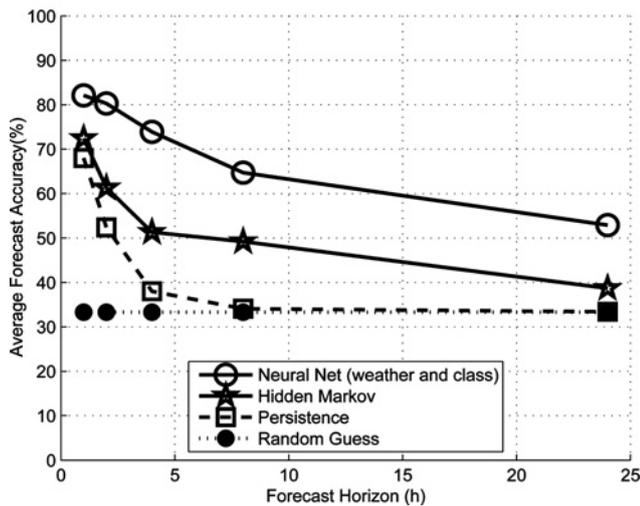
Fig. 6 Average forecast accuracy against horizon for three forecasting methods.
