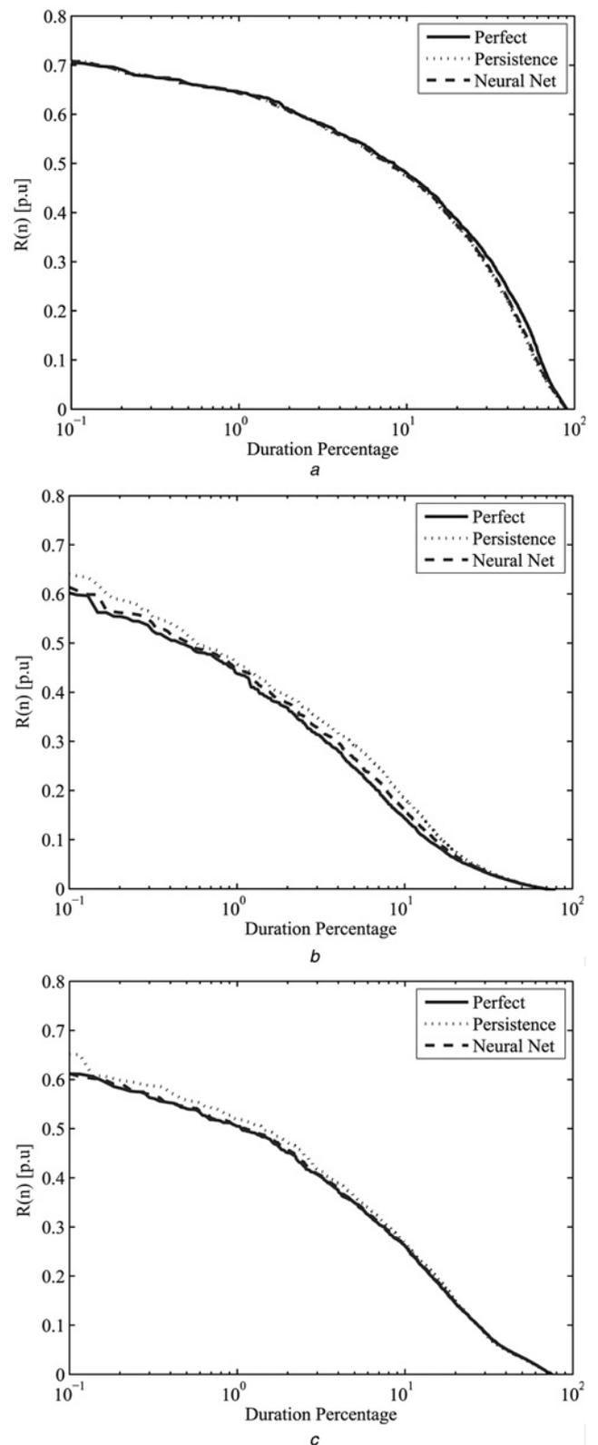
**Fig. 8** Reserve required for desired level of risks, ranging from 0.1 to 100%. Duration curves are for forecasted class types at a single site, compared with reserve required if knowledge of the class type was perfect
