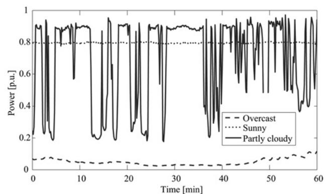
**Fig. 2** Examples of produced solar power by TU Delft 12.6 kW array for the three irradiance classes in June 2009
