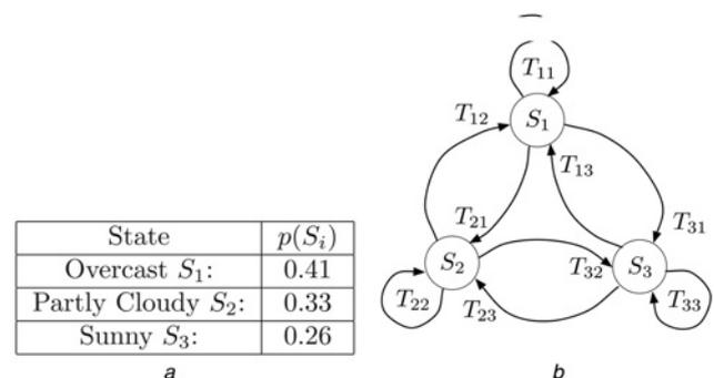
**Fig. 5** Probabilities associated with being in and transitioning between irradiance class states  $S_i$
