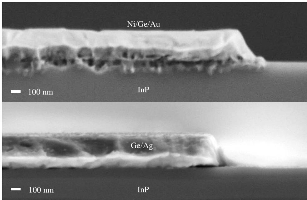
Figure 2. Cross-sectional SEM photos of metal/InP interface after annealing
