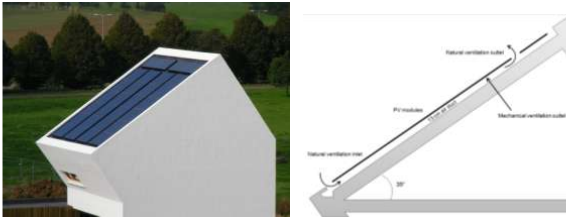
Fig. 3. and 4. PV field test in The District of Tomorrow consisting of 4 segments of PV modules and a vertical section of the field test with ventilation in and outlets providing different amounts of back-string ventilation.
