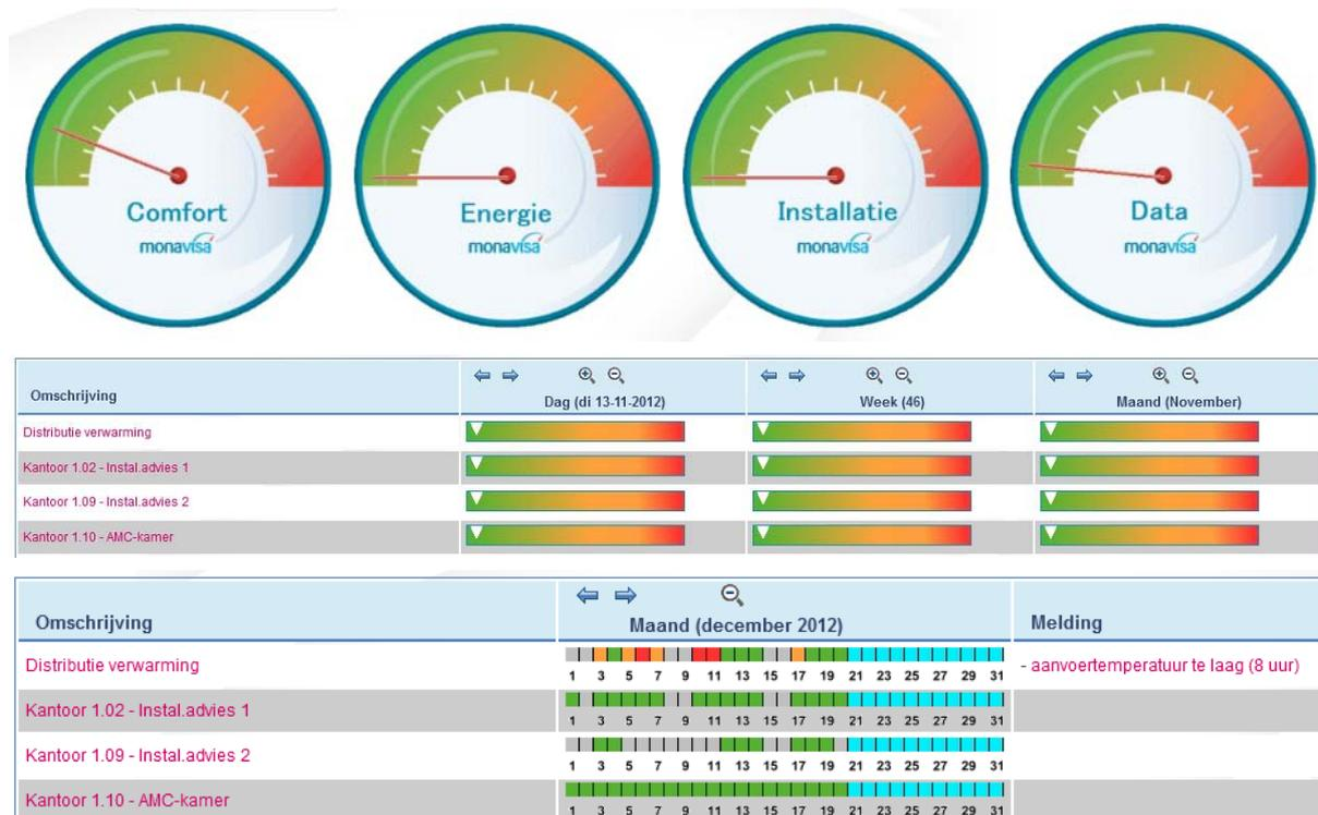
Figure 1. Monavisa interface and different levels of detail at which Monavisa shows information. From top to bottom: general overview for each category [Comfort, Energy, Building systems, Data availability]; overview for daily, weekly and monthly performance for each monitored room; detailed overview and assessment for each time interval and notifications for each monitored room [monavisa.dwa.nl].
