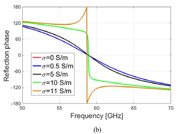
Fig.3. Calculated reflection characteristics with different conductivity by analytical expression. (a) Reflection magnitude. (b) Reflection phase.
