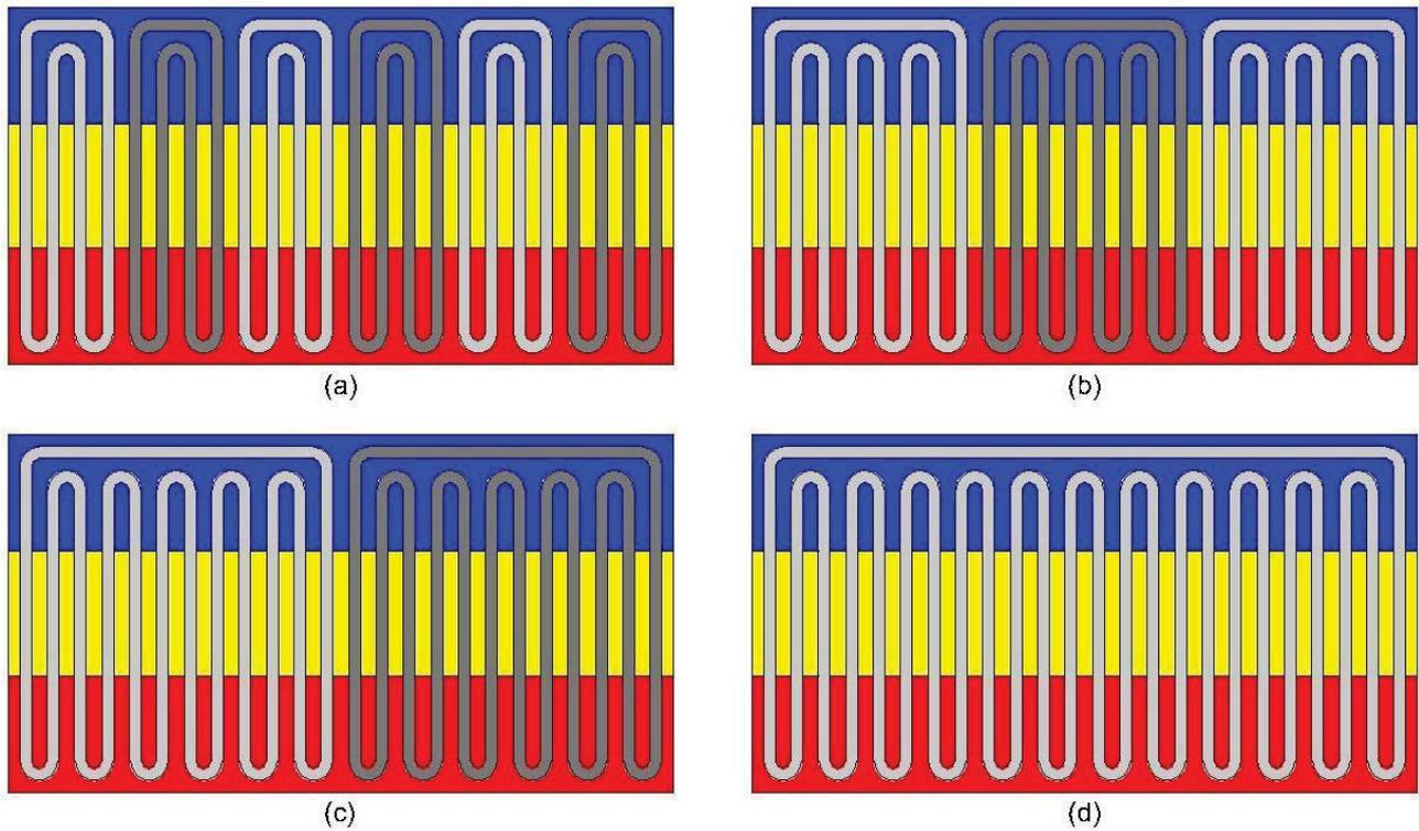
**Figure 2:** Different configurations: (a) six PHPs with two turns, (b) three PHPs with four turns, (c) two PHPs with six turns and (d) one PHP with twelve turns. Dimensions of the each configuration are given in Table 1.
