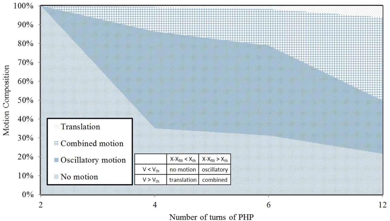
**Figure 4:** Motion composition in PHPs with different number of turns. The criteria for the different types of motion are indicated by the insert and explained in more detail in section 3.2.
