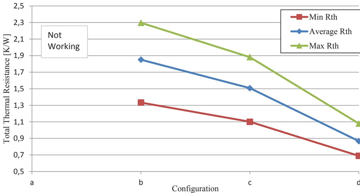
**Figure 3:** Total thermal resistance vs different configurations (See Fig. 2). The *blue line* shows the average thermal resistance of each configuration. *Green and red lines* show the maximum and minimum values for each configuration, respectively. The total heat input is kept the same for each configuration:  $Q_{in,tot} = 48W$ .
