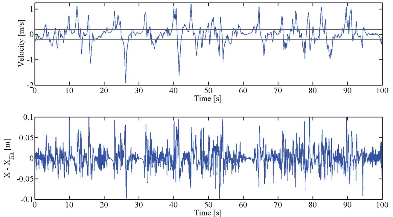
**Figure 6:** *Top:* Time derivative of the filtered displacement data as a function of time. If the velocity value is between the upper and lower thresholds,  $v_{th} = 0.2\text{m/s}$  and  $v_{th} = -0.2\text{m/s}$  respectively, the liquid slug is considered to be oscillating. *Bottom:* Difference between sampled data ( $X$ ) and filtered data ( $X_{filt}$ ) as a function of time. If the amplitude is smaller than threshold  $x_{th} = 10^{-2}\text{m}$ , there is no oscillation in the system.
