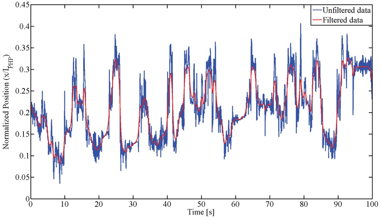
**Figure 5:** Normalized position of a liquid slug as a function of time. The *blue* and *red line* represent unfiltered and filtered displacement data, respectively.
