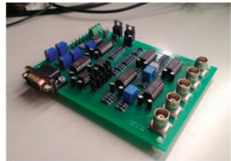
Fig. 12: An Electric Hindmarsh-Rose neuron
