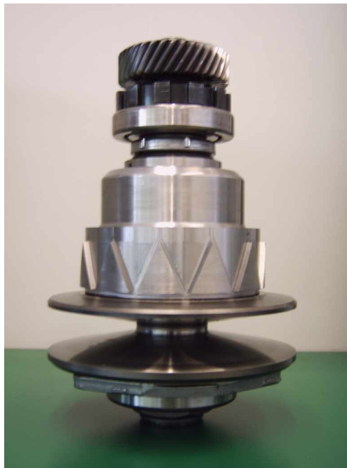
Figure 4.1: The new cylinder mounted on the secondary shaft
