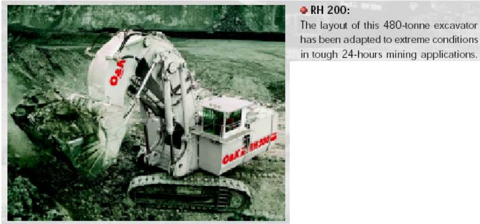
Figure 1.1 O&K RH200 hydraulic excavator in operation (From “ Mining Hydraulic Excavators ”, Terex Mining)
