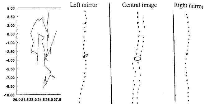
Figure 7: The path of a type III bubble filmed with high-speed camera.  $D_{tube} = 90$  mm,  $v_{s,l} = 0.25$  m/s,  $D_{eq,b} = 10$  mm. Left: dimensions in mm, right: distance between lines in reality 90 mm.
