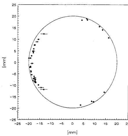
Figure 3: Wall-distribution.  $D_{tube} = 40$  mm,  $v_{s,l} = 0.20$  m/s,  $D_{eq,b} = 2$  mm.
