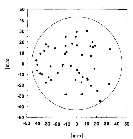
Figure 5: Spread-out distribution.  $D_{tube} = 90$  mm,  $v_{s,l} = 0.0$  m/s,  $D_{eq,b} = 6$  mm.
