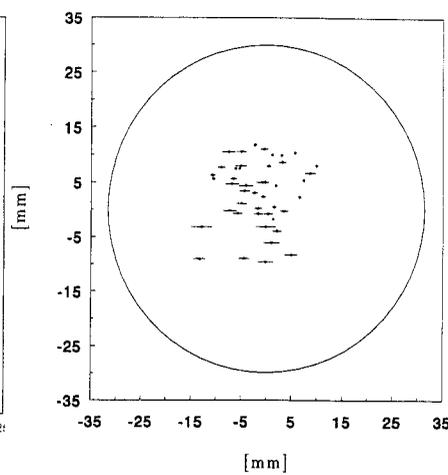
Figure 4: Central-distribution.  $D_{tube} = 60$  mm,  $v_{s,l} = 0.25$  m/s,  $D_{eq,b} = 0.9$  mm
