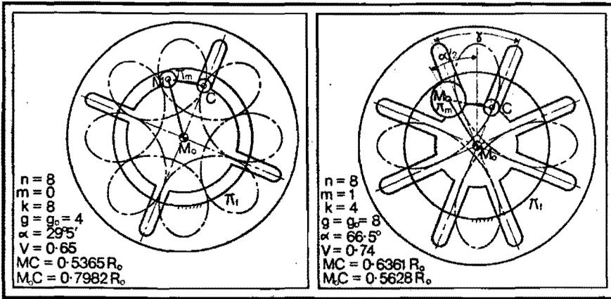
10, 11: Two hypocycloid gear-driven Geneva mechanisms
