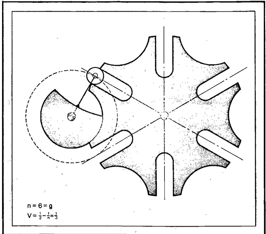
Design of a mechanism to give intermittent motion often relies on the conventional Geneva wheel. Here we describe the gear driven version of this mechanism, which gives a smoother transmission of power and permits input and output shafts to be coaxial
