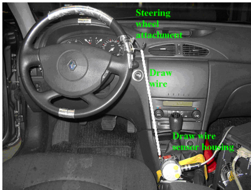
Figure 4.1: Steering wheel angle instrumentation
