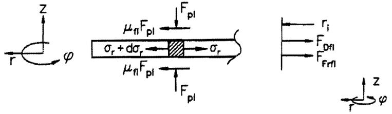
Figure 4: Forces on the flange
