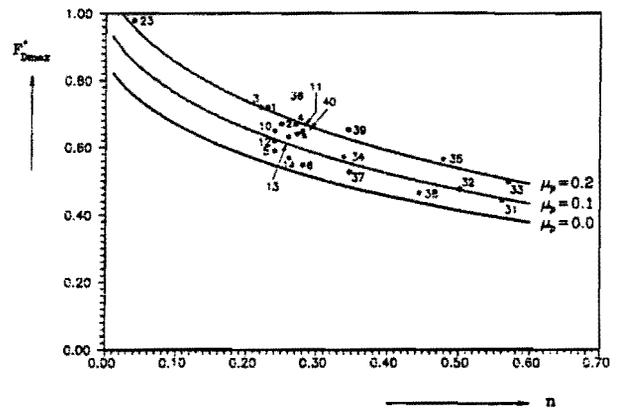
Figure 8: The maximum deepdrawing force vs strain hardening exponent  $n$ , with  $\rho_D/s_0 = 4$ ,  $\epsilon_0 = 0$ ,  $R = 1$ ,  $\beta_0 = 2$  for different materials
