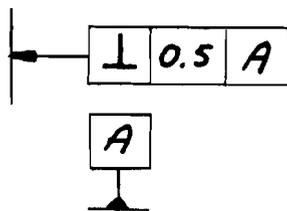
This indicates that the concerning plane should be perpendicular to plane A within a tolerance of 0.5 mm (for example see drawing E8502-01/B).
