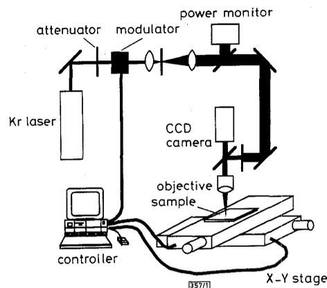
Fig. 1 Configuration of laser-beam writing system
