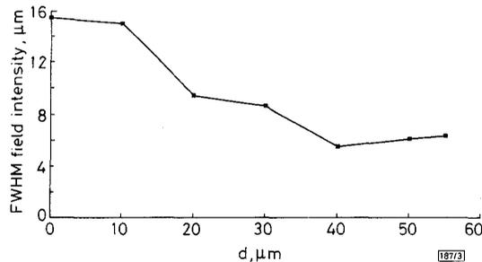
Fig. 3 Beam waist (FWHM) of intensity against propagated distance in air for structure of Fig. 1c
