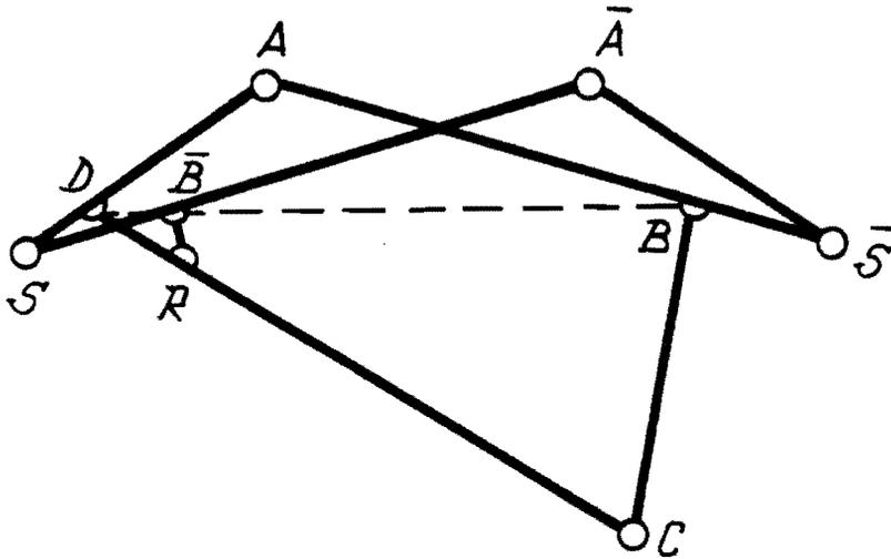
*Contraparallelogram-linkage adjoined with a linkage-dyad BCD and a bar  $\overline{BR}$  to overcome its stretched positions*
