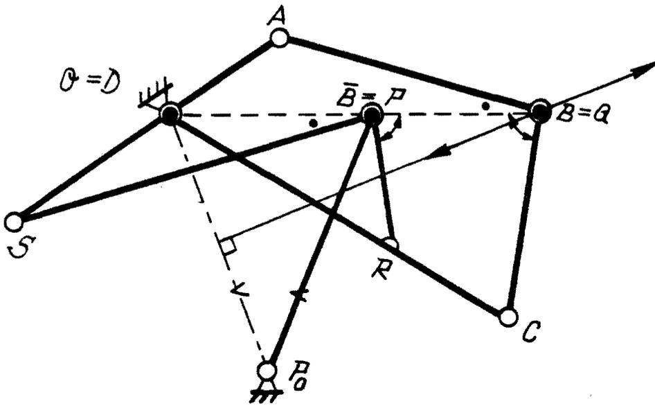
New Inversor with Q tracing a straight-line -segment.
