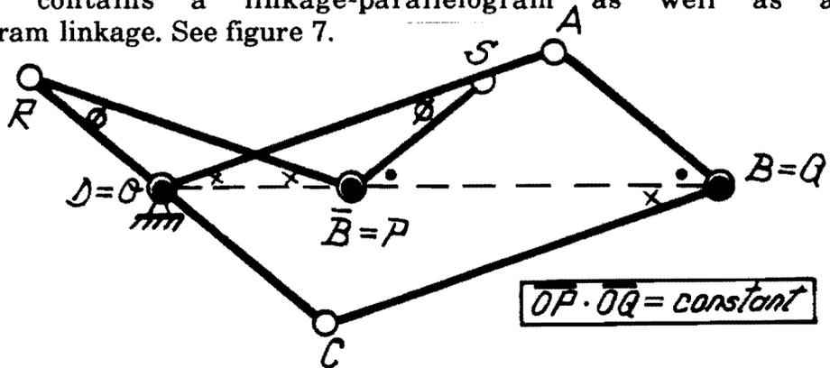
Particular *inversion-cell* with ABCD being a parl.gram-linkage
