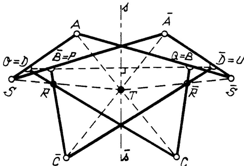
Two *perspective* contraparallelograms interconnected by the aligned joints  $D, \bar{B}, B$  and  $\bar{D}, \bar{B}$ , resulting into the *reflected* four-bars  $ABCD$  and  $\bar{A}\bar{B}\bar{C}\bar{D}$ , being interconnected by the joints  $S, R, \bar{R}$  and  $\bar{S}$
