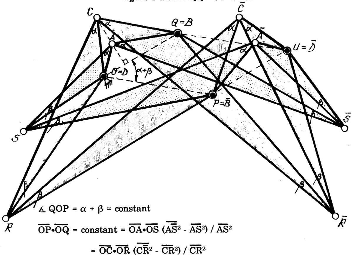
Two different quadruplanar *inversion-cells* of Sylvester and Kempe *interconnected* through 4 turning-joints Q, O, P and U, forming a parallelogram with variable lengths. Double overconstrained 8-bar linkage with two contraparallelogram-linkages, to wit  $AS\bar{A}\bar{S}$  and  $CR\bar{C}\bar{R}$ . Figure 9.
