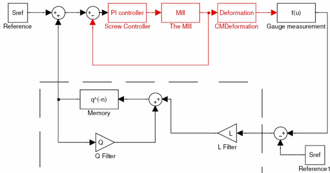
Figure 4. Feedback Loop and ILC Feedforward Loop
