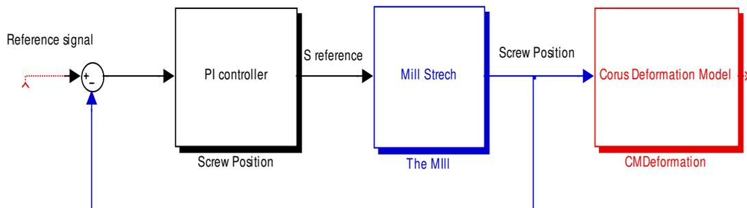
Figure 3. Offline Simulation Model
