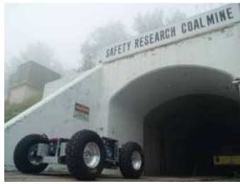
Figure 12: Mine Rescue Robot. Cave Crawler, courtesy The Robotics Institute, Carnegie Mellon University ( http://www.ri.cmu.edu/ )
