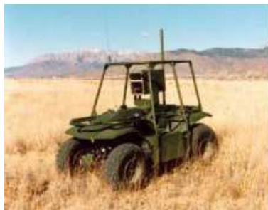
Figure 4: Unmanned Ground Vehicle. The Surveillance And Reconnaissance Ground Equipment(SARGE), courtesy Sandia National Laboratories ( http://www.sandia.gov/isrc/SARGE.html )
