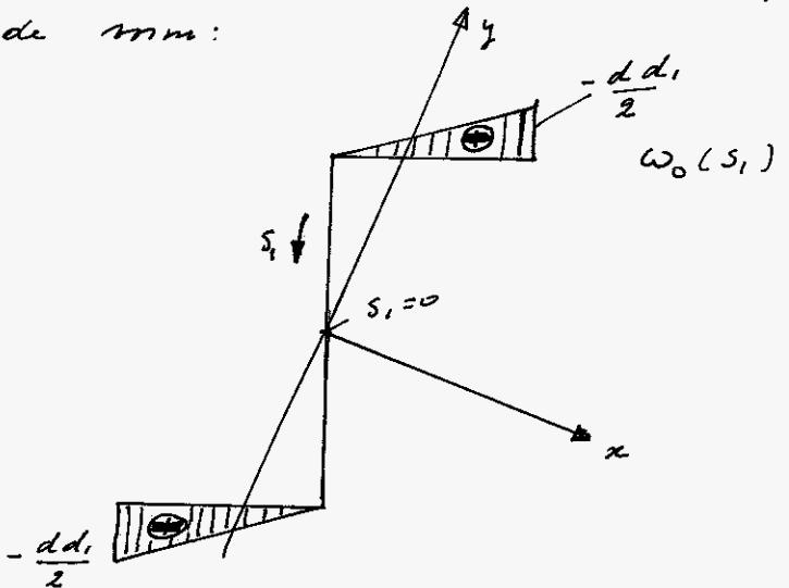
$$\begin{aligned} \int_{\text{F}} w_0 y \, dF &= 0 \\ \int_{\text{F}} w_0 x \, dF &= 0 \end{aligned} \quad \left\{ \begin{array}{l} \text{Dus } a_x = 0 \\ a_y = 0 \end{array} \Rightarrow \boxed{A = 0} \right.$$
