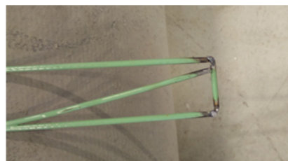
Figure 2 Welded end of the bed joint reinforcement forming a loop.
