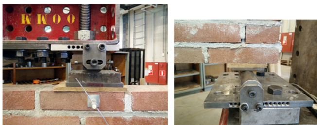
Figure 4 Load introduction point and support, soft board and steel platen used to spread the load evenly.
