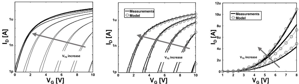
**Fig. 5a:** Transfer characteristics measured with  $V_{TG}$  in the range  $\{-5,5\}$  and a step of 1 V, increasing in the direction of the arrow. **5b:** Detail of negative  $V_{TG}$  measurements and simulations: a threshold modulation is observed. **5c:** Measurements and simulations for positive  $V_{TG} = 0; 2; 5$  V: an on-current modulation is observed.
