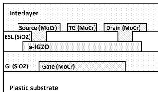
**Fig. 1:** Cross section of an a-IGZO TFT. The layer stack is formed as follows (from the bottom): Plastic substrate, gate metal, gate insulator (GI), a-IGZO, ESL, source/drain metal, and final insulator (interlayer).
