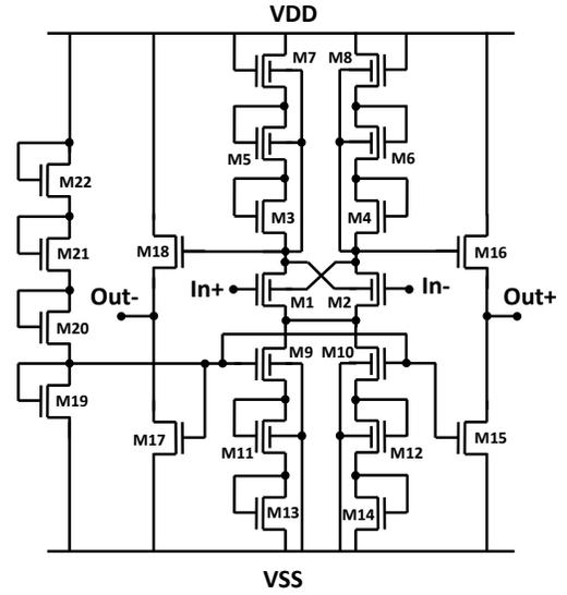
**Fig. 8:** Amplifier with positive feedback and a load circuit (M<sub>3</sub>, M<sub>5</sub>, and M<sub>7</sub>) which drastically improves DC gain.
