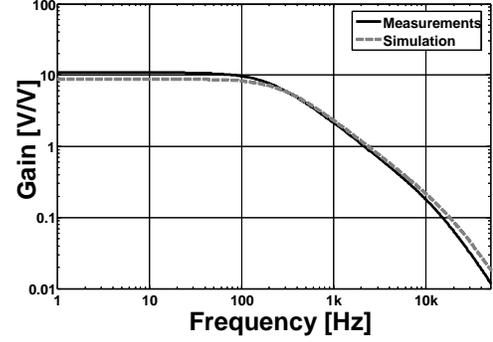
Fig. 12: Frequency response of the circuit in Fig. 7
