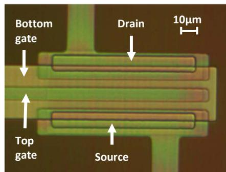
**Fig. 2:** Picture of a fabricated double gate TFT.
