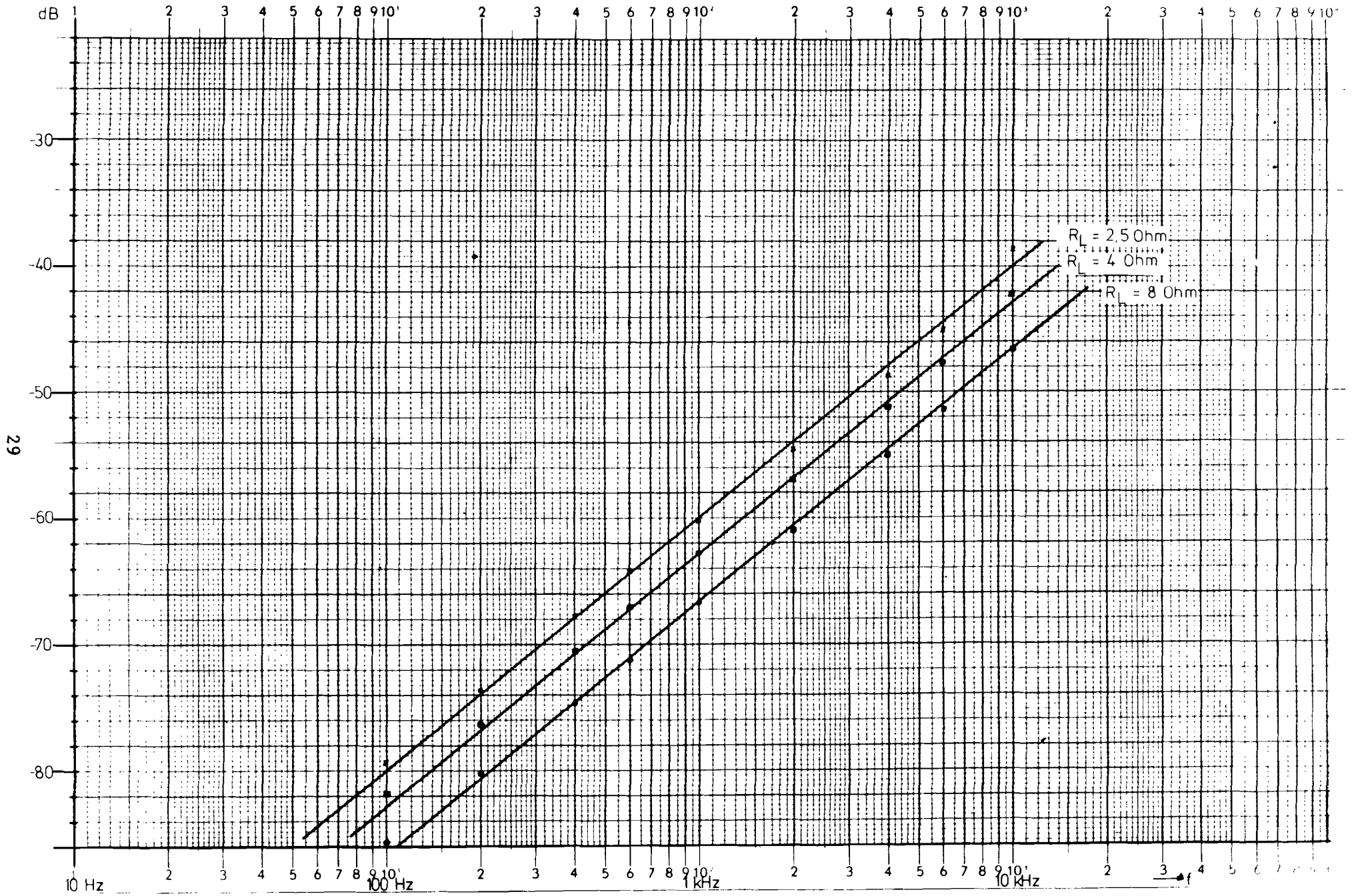
Fig 4.12 d = d(f) metingen. A_{10} f_{11} = 1 \text{ MHz} . k_{10} = 1 . g_{m1} = 0,25 \text{ S} .
