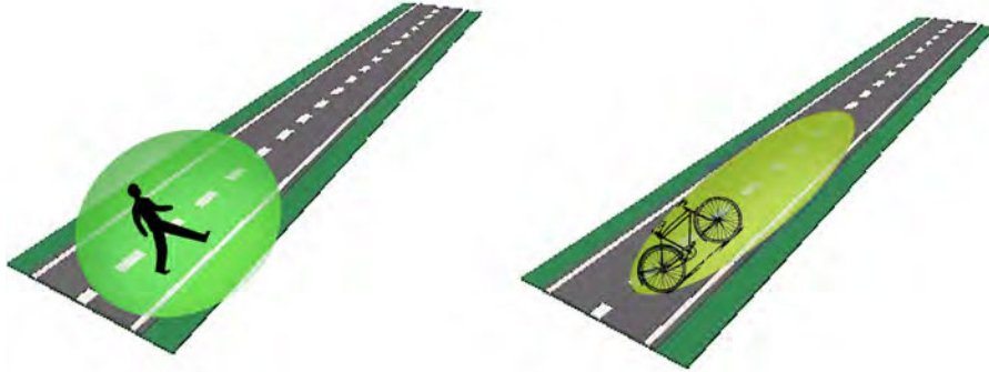
Figure 2.2: Schematic drawing showing the difference in immediate environment for pedestrians (left) and cyclists (right).
