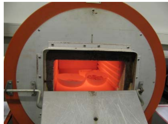
Figure 25: Heated fly ash in oven at 800°C
