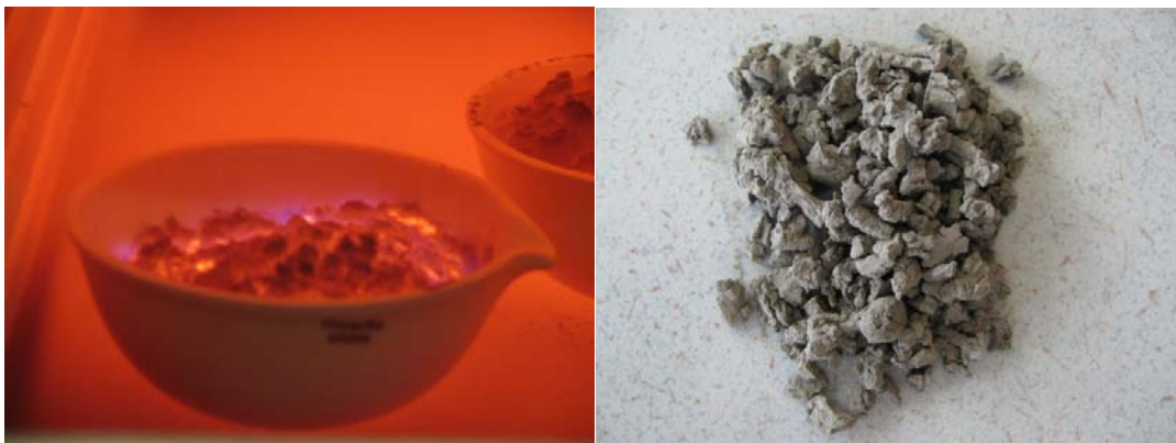
Figure 49: Thermal treated HVC filter fly ash after one hour in oven at 750 degrees Celsius
