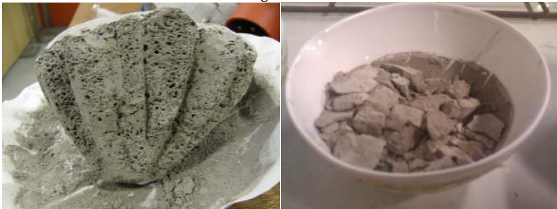
Figure 48: Fixed HVC filter fly ash (left) and HVC cyclone fly ash (right) due to cementitious properties
