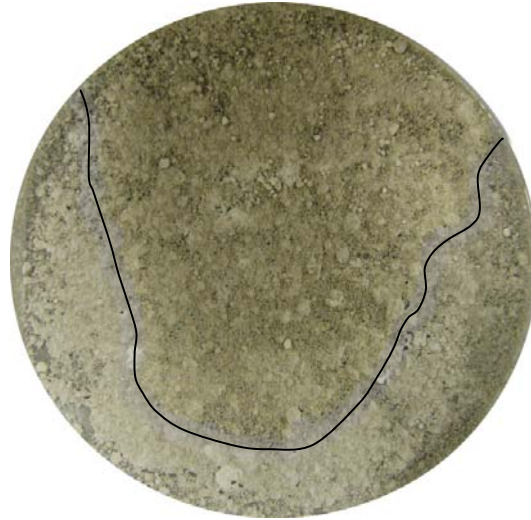
Figure 10: Comparison original (light region) and water treated (dark region) paper sludge fly ash separated by a dark line surrounded with a white glow.
