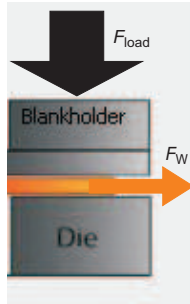
Figure 1.2: Macroscopic forces in the blankholder region.
