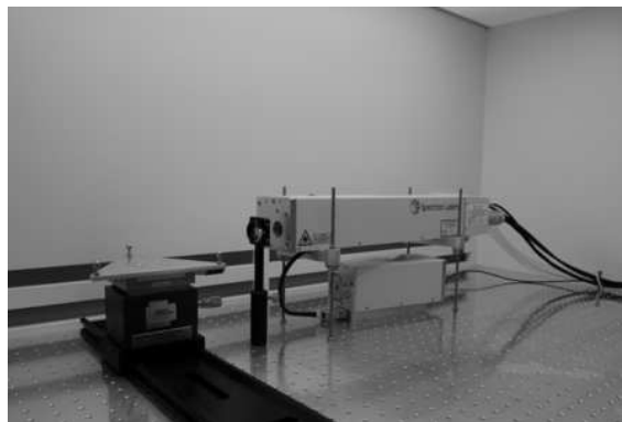
Figure 5.1: Picture of the LSC setup that was used for the cleaning experiments. The setup consists of a Q-switched Nd:YAG laser, a single plano-convex \text{CaF}_2 lens, and a micrometer controlled xyz-stage.
