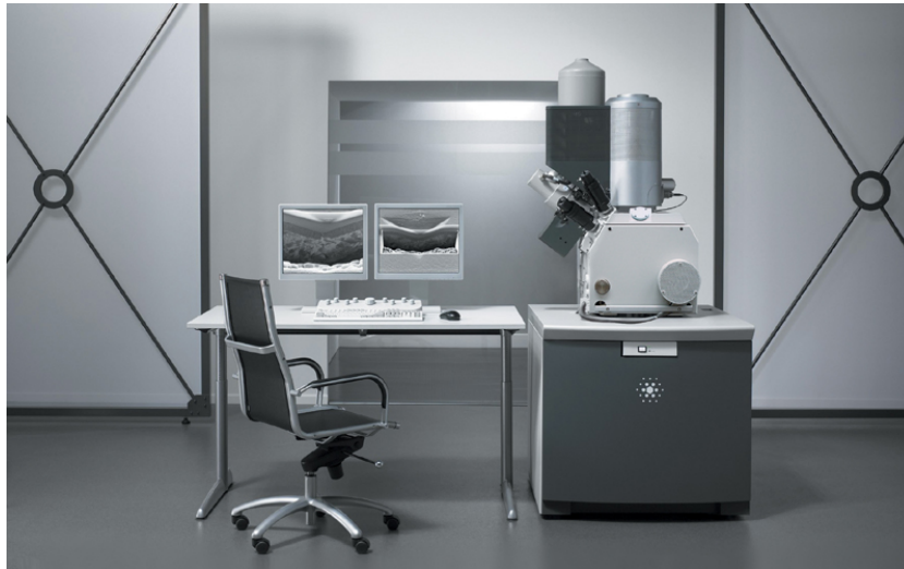
Figure 6.1: Picture of a typical Focused Ion Beam (FIB) system. This system is a FEI Company Nova600 DualBeam in which also a scanning electron microscope is incorporated.
