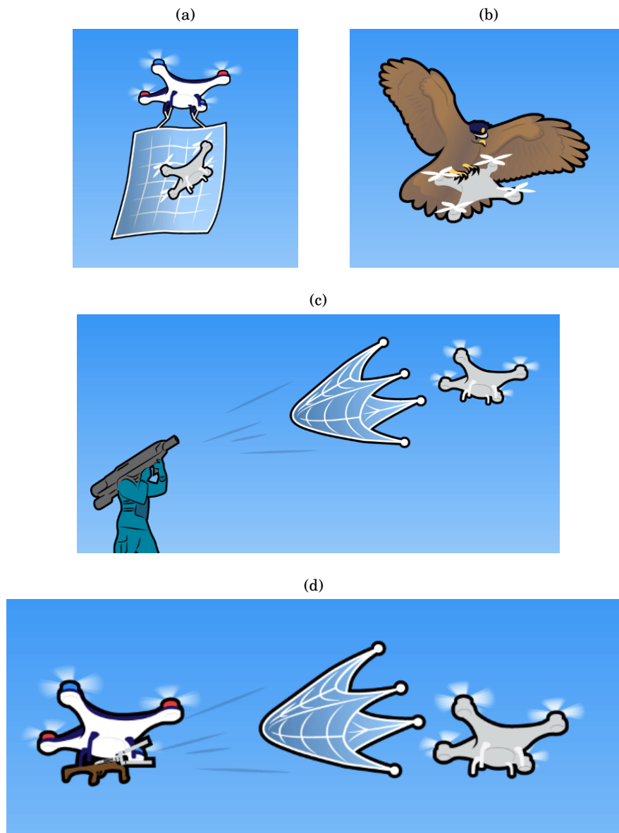
FIGURE 1.1. (a) Japanese police. Drone catching another drone using a net.(b) Dutch police. A hawk catching a Drone. (c) Openworks Engineering. A gun to shoot a net (d) Michigan Tech. Combination of a net gun and a drone
