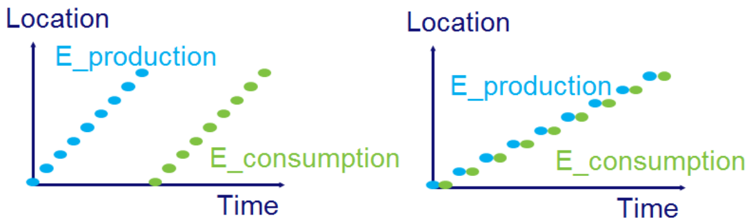
Figure 3-5 Improvement of data locality for array E in 3mm a) original b) after loop fusion
