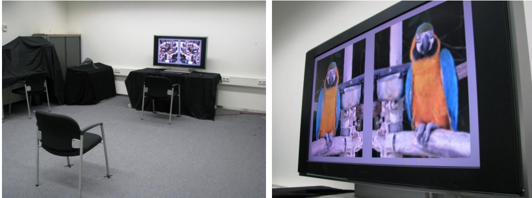
Figure 12 The setup for the JND experiment consisted of a TV which could be viewed at different environmental conditions.
