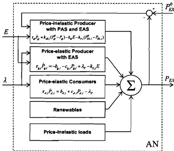
Fig.3: Internal structure of autonomous network
