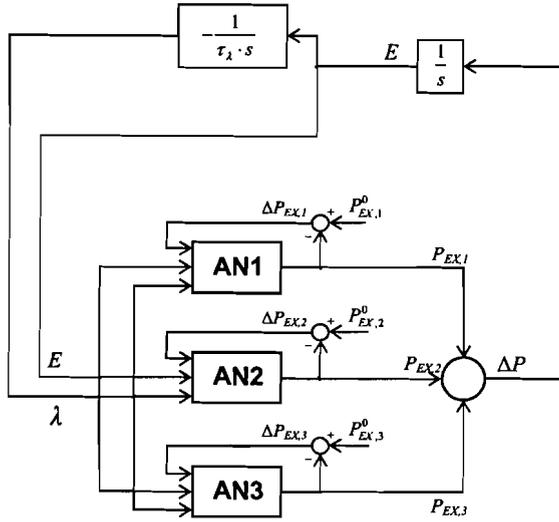
Fig. 2: AN Power system with decentralized control signals
