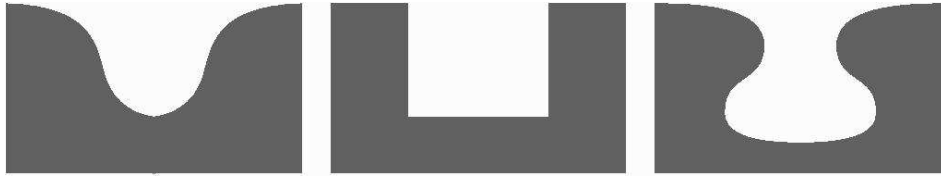
Figure 1.4: Different types of gratings: a non-overhanging grating (left), a binary grating (middle), an overhanging grating (right)
