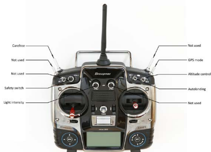
Figure 4.6: Graupner MX 20 HoTT remote controller channel configurations
