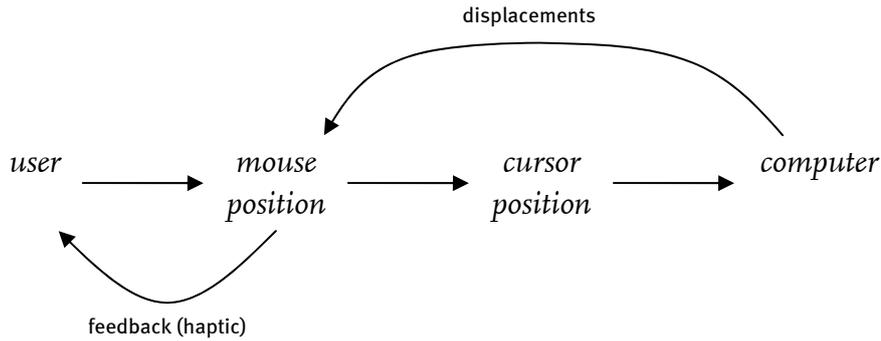
**Figure 2: Force-Feedback mouse feedback loop**
