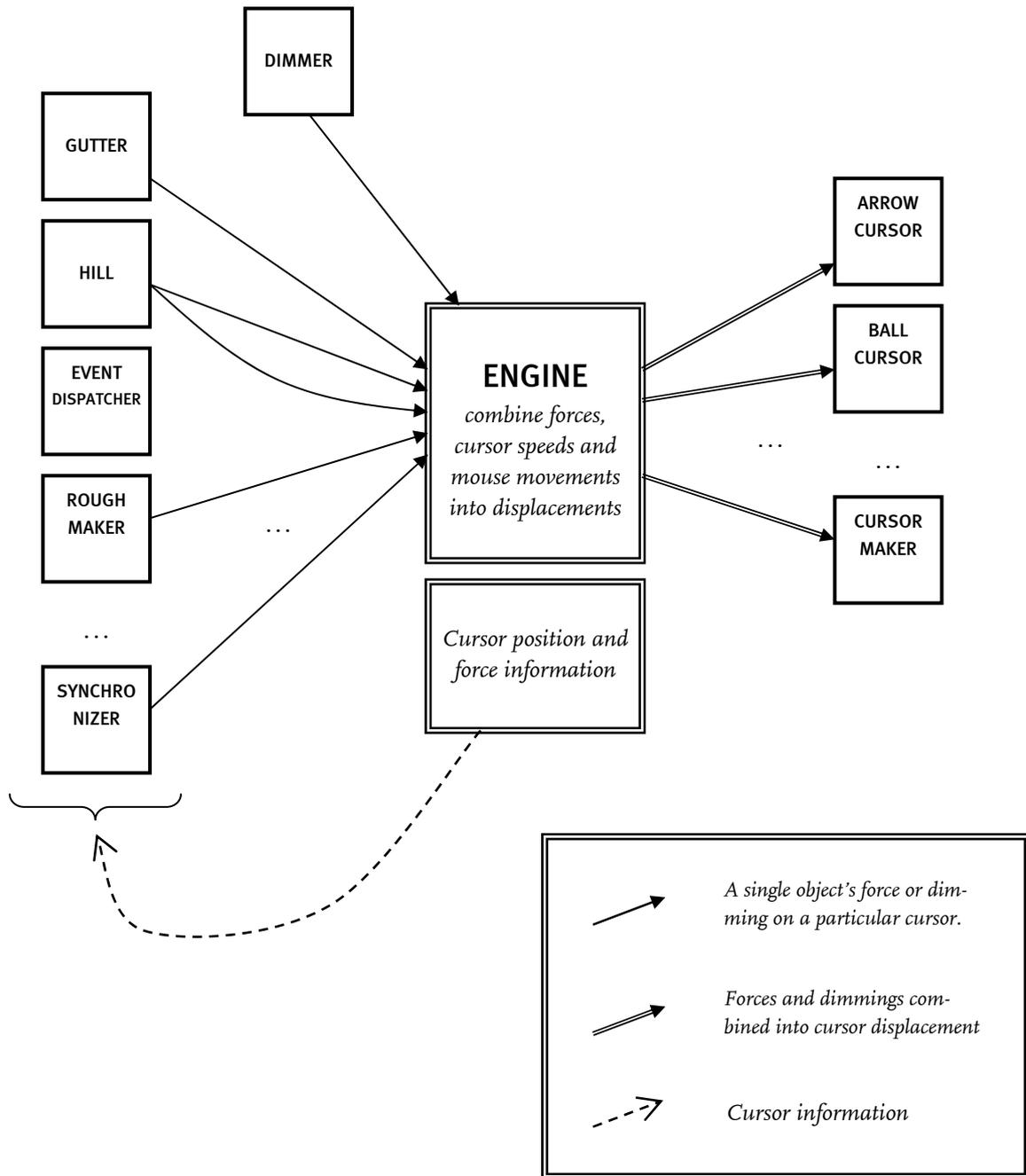
Figure 6: Calculation of cursor displacements through the different PowerCursor objects.
