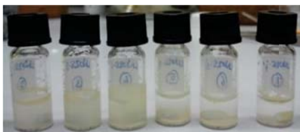
Figure 4.9: Various catalysis samples after 24h reaction time showing the inhomogeneous nature of the samples.
